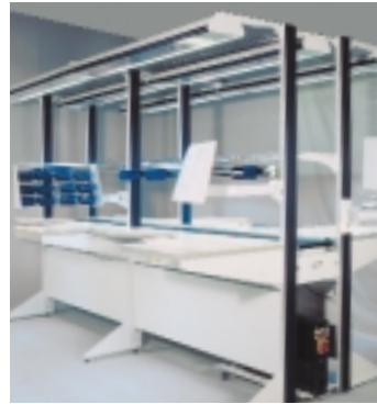
JOT Automation flat belt conveyor, PLC controlled, circuit board assembly operation.
